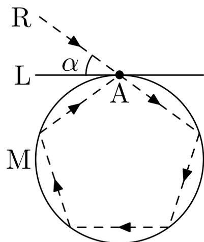
M is a circular mirror with a reflecting surface on the inside; A is a small hole in M with a semi-transparent detector (light may come in but not go out); R is an incoming ray of light;  $\alpha$  is the angle between R and the horizontal plane L.
